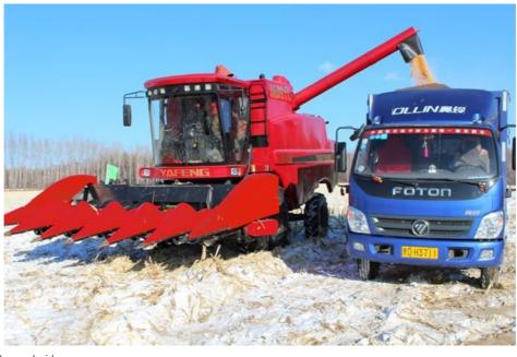
Picture 1: Self-propelled corn kernel harvester
